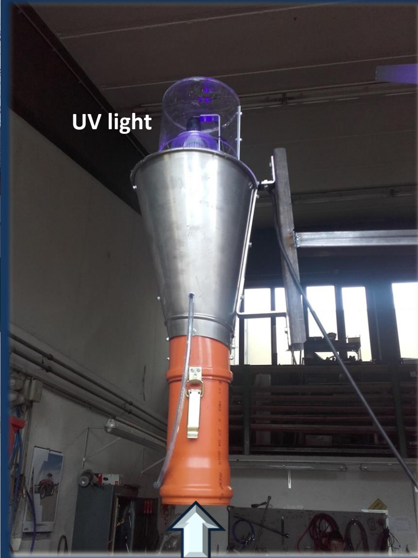
Net inside to catch the insects & insecticide stripe
